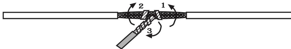
6. Use electrical tape to wrap. Be sure to cover the wire about two inches on either side of the connection. First pull the wire that you have just connected along side the wire you connected to, tape and wire tie them together. Use this method for all connections.
