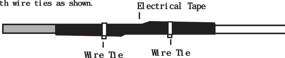
Use this method **ONLY** when connecting two separate wires end to end.
