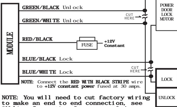
**NOTE:** You will need to cut factory wiring to make an end to end connection, see "Making Connections" on pages 3-4.
