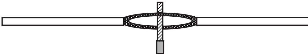
5. Wrap the wire around one side then the other and finally around itself as shown.
