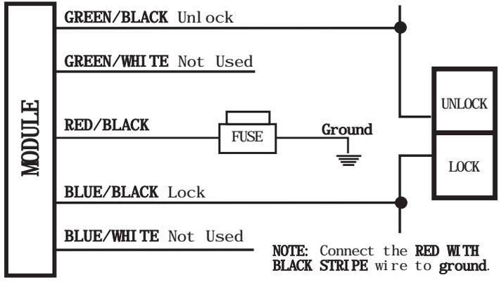
**NOTE:** Once you have made the connections for the 5-pin door lock harness, you will need to plug the door lock harness into the main module 5-pin plug on the front of the unit.
