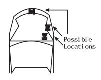
Step 2: Use three self-tapping screws (included) to secure the alarm. Screw into a well-grounded metal surfaces. **CAUTION: You must use all three screws.**
