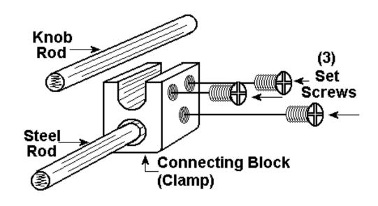
Fig. 4 Set-up for Correct Travel on ACTUATORS
